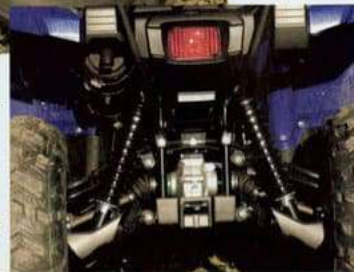
(above) Yamaha's EPS preserves a measure of feedback through the bars, but masks rim- and tire-damaging obstacles. (right) It may be set too soft from the factory, but Yamaha's adjustable suspension is a big benefit for work or recreational riding.
